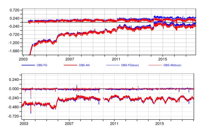
The lower panel shows the same time series for AIRS 787 in ERA-5 where the bias initialisation problem was addressed. There is now no evidence of a drift in this channels and it is believed that this is a much more realistic representation of the excellent stability of this channel and the AIRS instrument in general.
