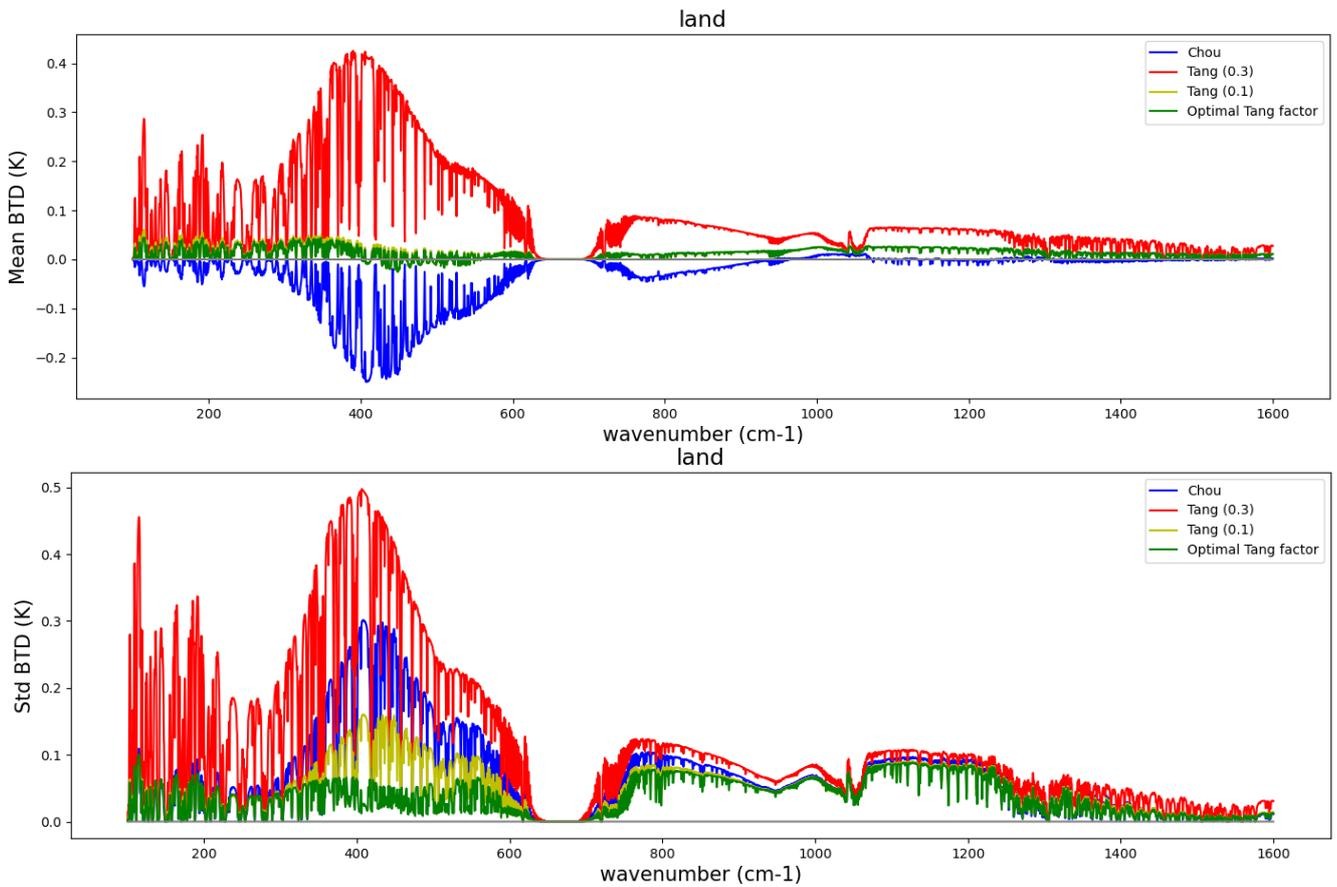
Figure 1: Mean (top) and standard deviation (bottom) of the difference between DOM computation and the Chou scaling approximation (blue line), the Tang correction with TangFact = 0.3 (red line), the Tang correction with TangFact = 0.1 (yellow line) and the optimal Tang factor (green line).
