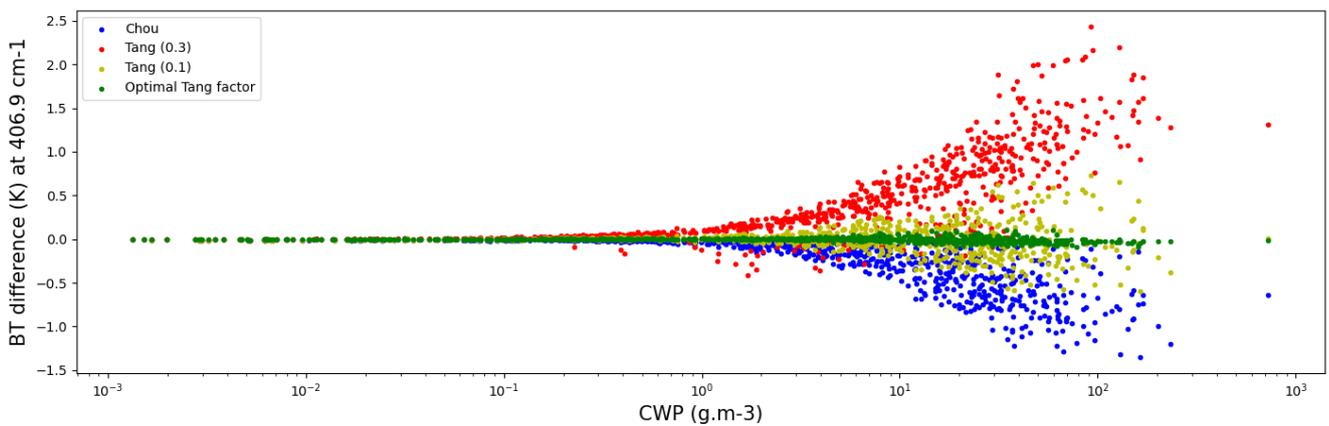
Figure 4: Brightness temperature difference at  $406.9 \text{ cm}^{-1}$  between the DOM computation and the Chou scaling approximation (blue dots), the Tang correction with TangFactor = 0.3 (red dots), the Tang correction with TangFactor = 0.1 (yellow dots) and the optimal Tang factor (green dots), as a function of the cloud water path (CWP)
