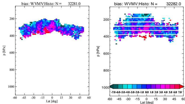
Figure 4.5: Zonal mean obs-fg bias [m/s] for simulated water vapour clear-sky AMVs with histogram height assignment. An  $QI$  threshold of  $>60$  is always applied. In the ‘raw’ data (left) only those AMVs are considered that are also present in the ‘final’ data set (right).
