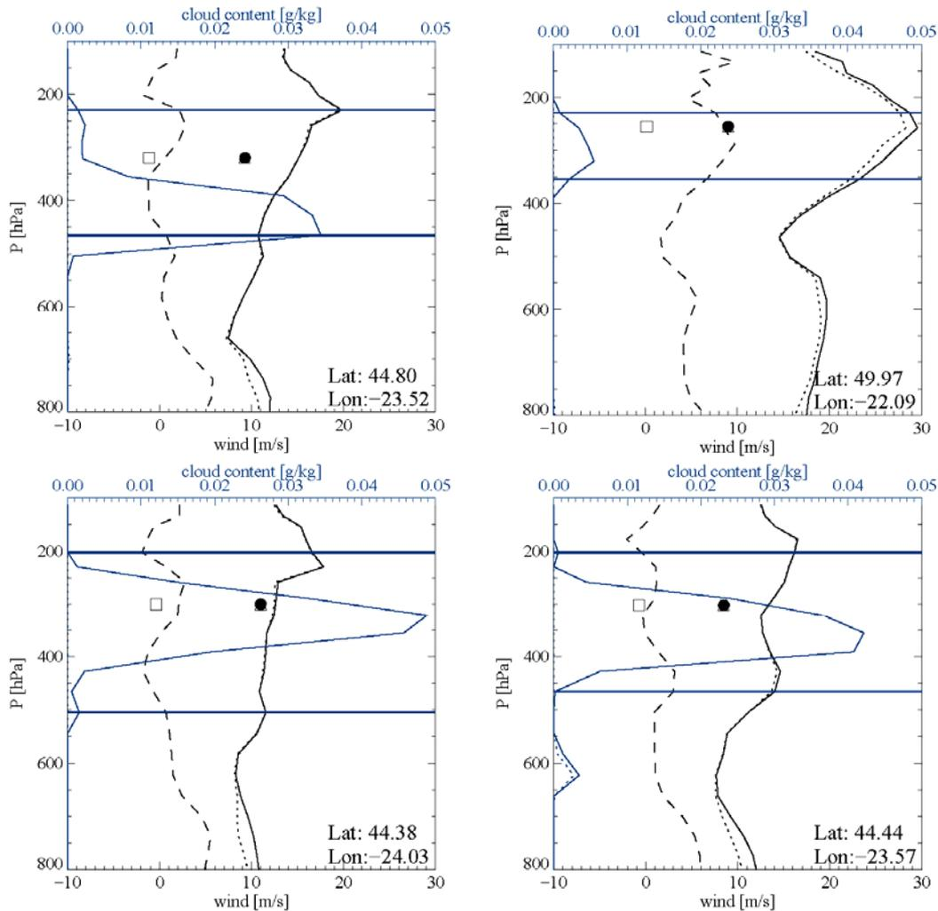
Figure 6.1: Examples of cirrus clouds (solid blue line) as cloud content profile [g/kg]. The model wind speed profile is solid and  $u, v$  components are dashed and long-dashed, respectively. The diagnosed range of cirrus cloud is marked by two horizontal lines. The AMV observation (IR,  $H_2O$  intercept method) is shown as bullet, triangle and square, respectively for wind speed,  $u$  and  $v$  component.
