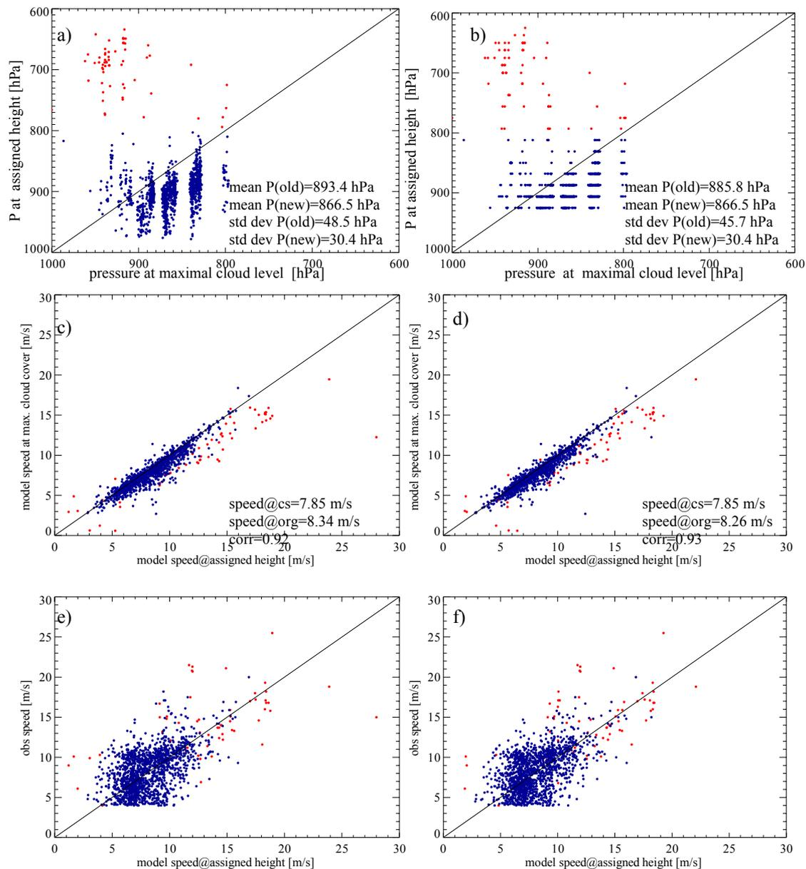
Figure 5.4: Extracted cases with low inversion clouds. Comparison of original assigned AMV observation versus model values at cloud base in terms of pressure (a, b) and wind speed (c-f). Results are shown for the raw quality data set (left column) and the final quality data set (right). Original observations above 800 hPa are marked in red.
