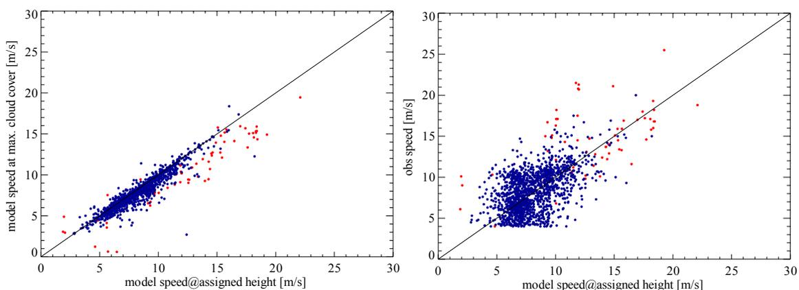
Figure 1.3: Extracted cases with low inversion clouds. Model speed at inversion cloud base (left) and observed AMV speed (right), respectively versus model speed at originally assigned AMV height (after auto-editing and  $QI > 60$ ).
