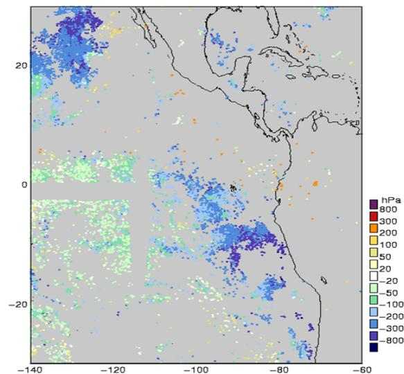
Figure 5.1: Pressure difference between the observed AMV pressure and model best-fit pressure for the unedited GOES-12 VIS winds at 3 July 2007 15 to 21 UTC. Note, the large AMV positive height bias (blue colours) off the coasts of Peru and Mexico. (Forsythe, 2008).
