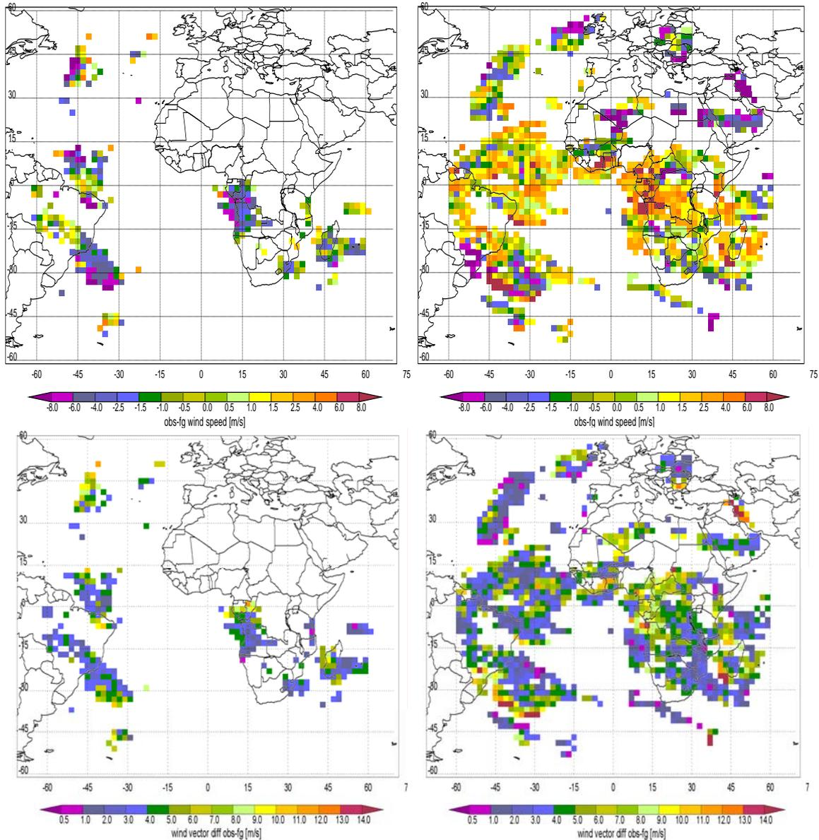
Figure 4.1: Bias (top) (obs-fg) and mean vector difference (bottom) of (final quality, NOGAPS background) simulated AMVs (left) and real Meteosat-8 AMVs from the 6.2 micron water vapor (cloudy) channel. The height interval is 200-300 hPa and the time period is 6 hours (2 Jan 2006 12-18UTC). Quality indicator threshold for simulated and real observations is 60.
