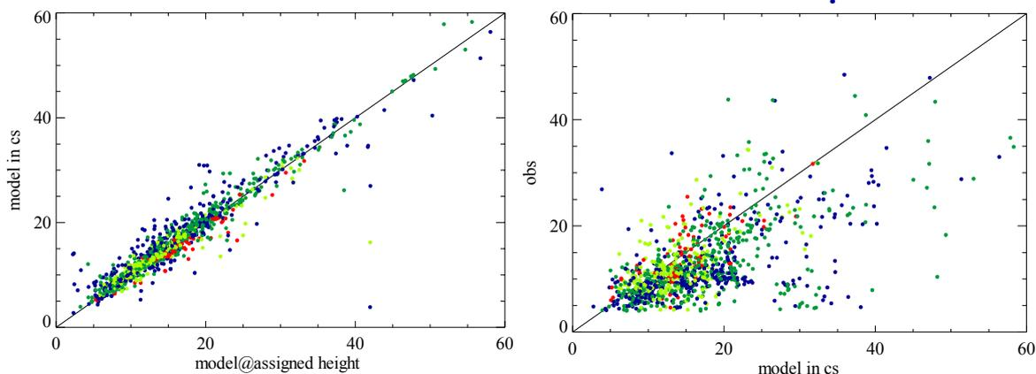
Figure 1.4: Mean model wind speed [m/s] in the cirrus cloud versus model speed at the originally assigned height for IR AMVs (left). On the right the observed AMV speed [m/s] is plotted versus the mean model wind speed in the cirrus cloud. The colour coding corresponds to the thickness of the cirrus cloud in terms of numbers of model levels. Blue, dark green, bright green, red is from thin to thick cirrus. (“raw” AMVs, i.e. before autoediting,  $QI > 60$ ).
