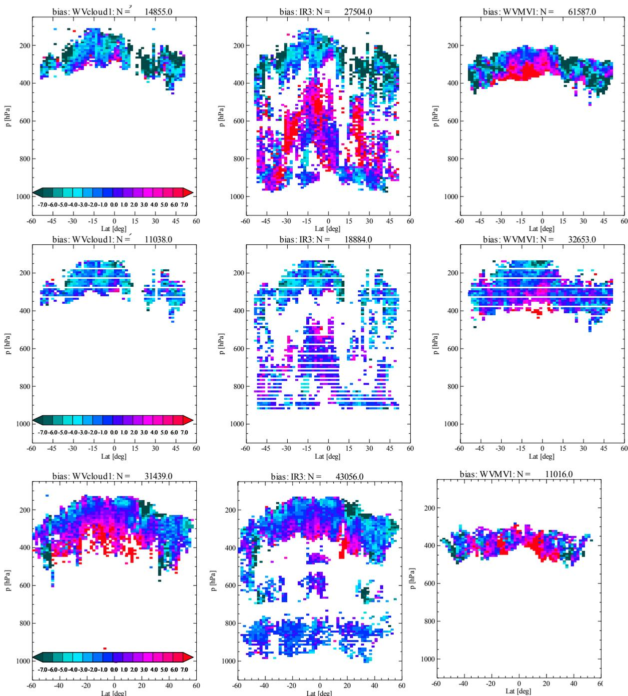
Figure 4.2: Zonal mean obs-fg bias [m/s] for simulated (*NOGAPS background*) AMVs (top, raw quality and middle, final quality) and real METEOSAT-8 AMVs (bottom) for 6.2 micron cloudy water vapor AMVs, 10.8  $\mu\text{m}$  IR AMVs and 6.2 micron clear water vapor AMVs. The time period is 2 Jan 2006 12-18UTC). Quality indicator > 60.
