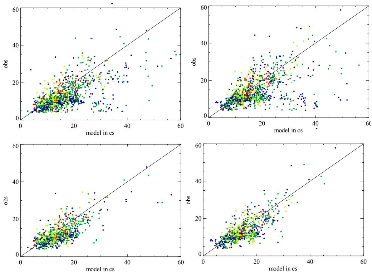
Figure 6.3: Observed AMV speed [m/s] versus model speed in idealized cirrus clouds for IR (left) and water vapour cloud (right) winds. In the upper figures all winds from the raw quality data set that passed the cirrus selection criteria are plotted. In the lower figures only raw quality winds that are found in the final data set are plotted.
