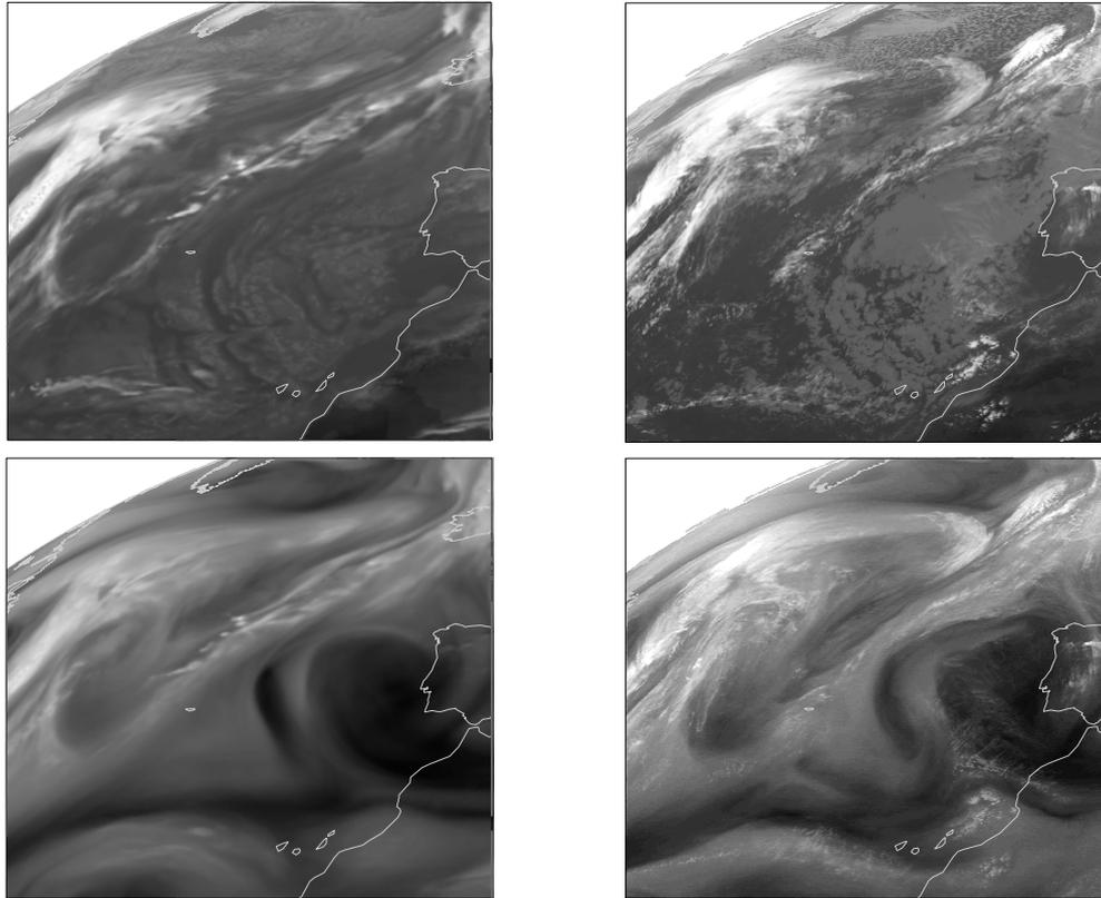
Figure 1.1: Simulated (left) and observed Meteosat-8 (right) IR  $10.8\mu\text{m}$  (top) and  $6.2\mu\text{m}$  (bottom) image (2 Jan 2006, 15.45UTC).
