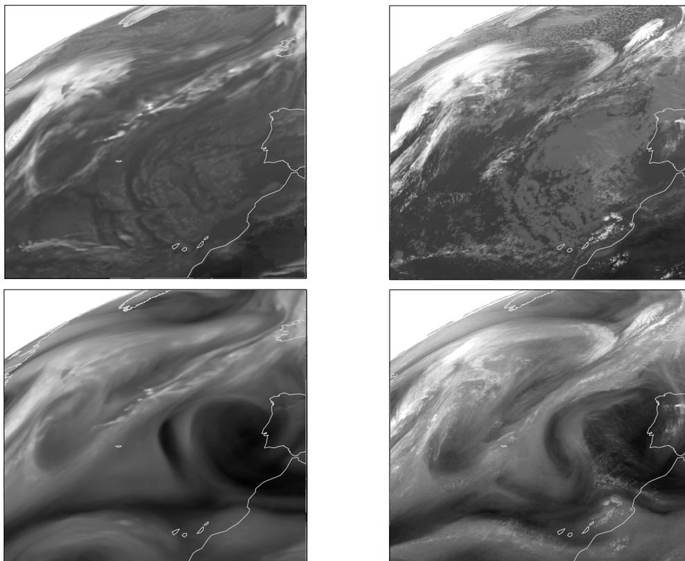
Figure 3.1: Simulated (left) and observed Meteosat-8 (right) IR 10.8 $\mu\text{m}$  (top) and 6.2 $\mu\text{m}$  (bottom) image (2 Jan 2006, 15.45UTC).
