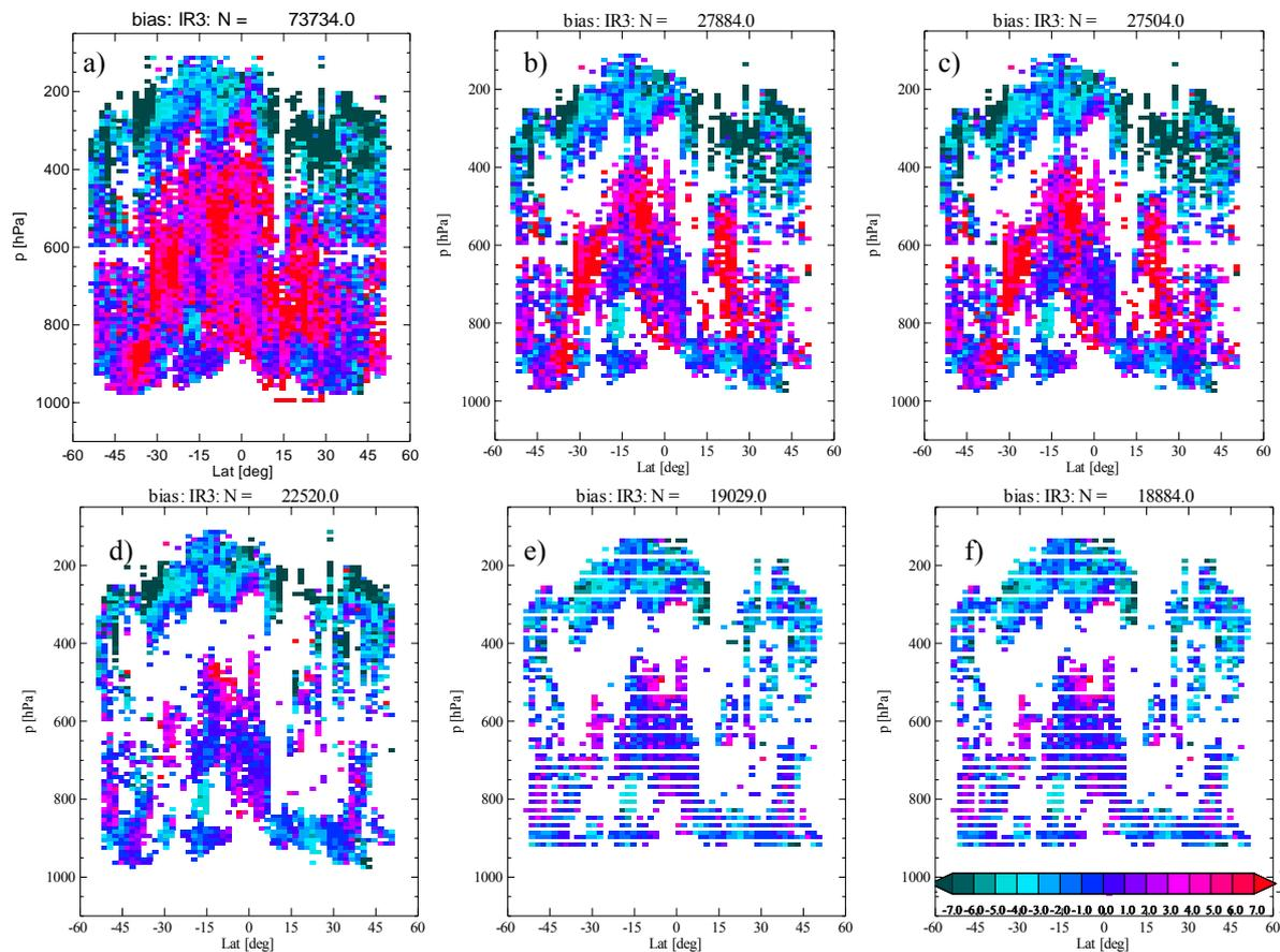
Figure 4.3: Zonal mean obs-fg bias [m/s] for simulated IR AMVs at various stages of the AMV post-processing. a) all derived AMVs (no QI filter), b) all derived AMVs, c) raw AMVs, d) checked AMVs, e) autoe AMVs and f) final AMVs. See text for details on different post-processing stages. QI>60 is applied in the last five figures.
