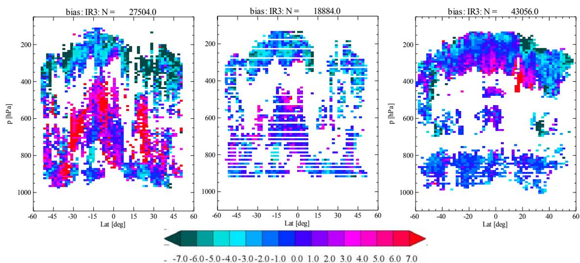
Figure 1.2: Zonal mean speed bias (AMV-truth, m/s) for simulated IR AMVs (left before auto-editing, middle after auto-editing) derived with the NOGAPS background. Also shown is the equivalent zonal mean speed bias for real Meteosat-8 AMVs (Jan 2006 12-18UTC). Quality indicator  $>60$ . Numbers at the top indicate the number of winds in the sample.
