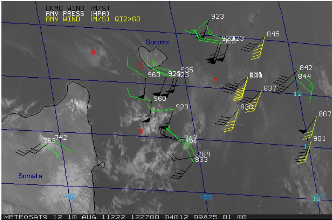
**Figure 21:** McIDAS visualisation of 1km Meteosat-9 high resolution visible imagery at 1227z over the tip of Somalia. Collocated Meteosat-9 high resolution visible AMVs (coloured by speed) and Met Office model winds (black) have been plotted along with the AMV assigned pressure. A long barb represents 5 m/s and a pennant 25 m/s. AMVs extracted at 1230z only.
