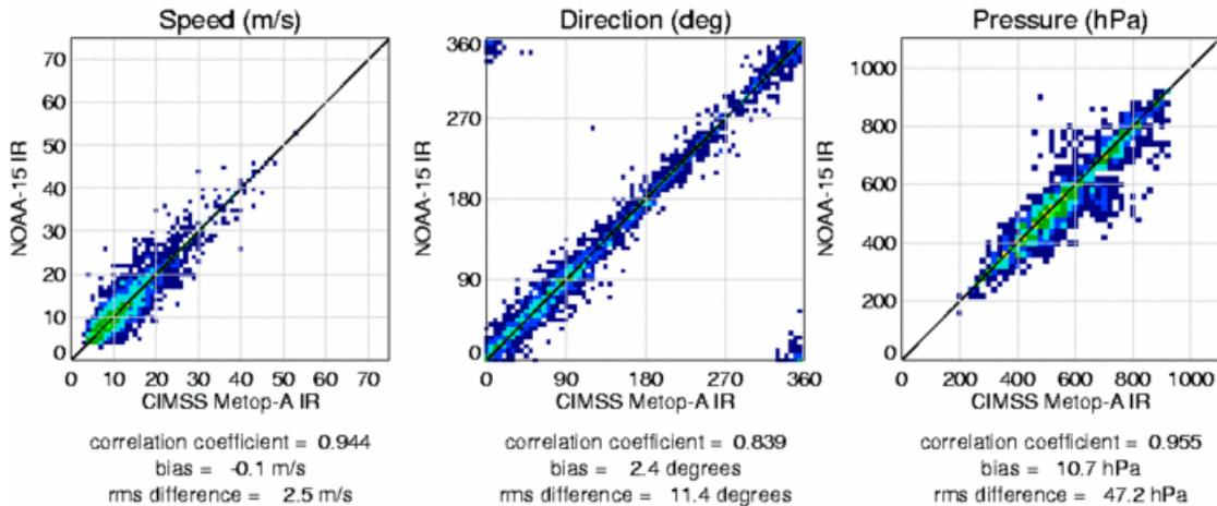
**Figure 5:** Collocation plots of speed, direction and pressure differences between NOAA-15 and Metop-A for December 2010. Observations were allowed to be up to 10 km apart and up to 30 minutes different in observation time. 4344 matches.
