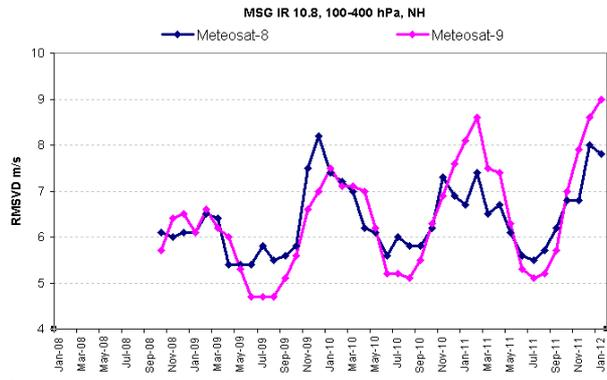
**Figure 31:** Time series of Met Office monthly CGMS statistics for Meteosat-9 and Meteosat-8 high level IR AMVs: root mean square vector difference for October 2008 to January 2012. Statistics calculated against the Met Office global model background for AMVs with Q11 > 80% (with first guess).
