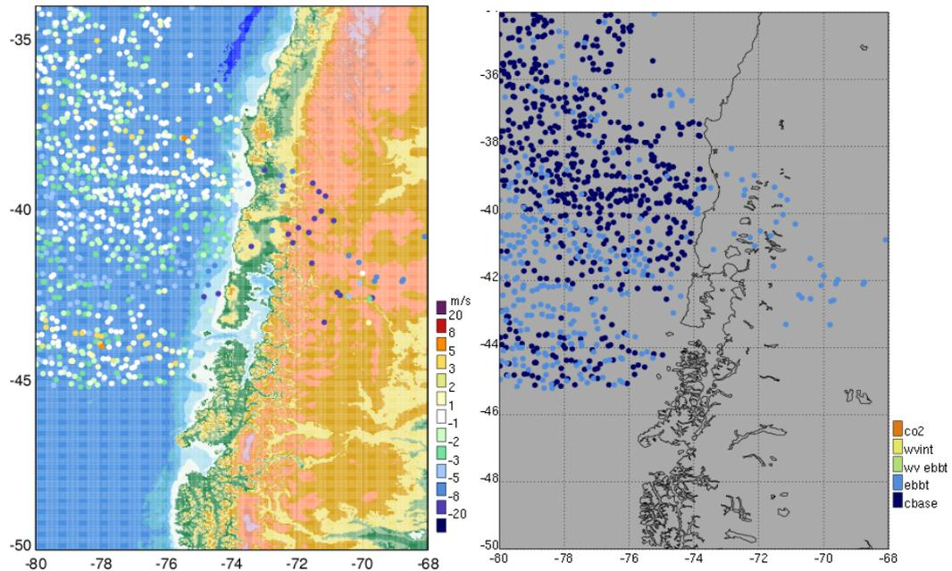
**Figure 15:** Maps of O-B speed difference with topography (left) and height assignment method (right) for GOES-13 visible winds. Data valid at 18z 19 December 2010 compared with the Met Office model background.
