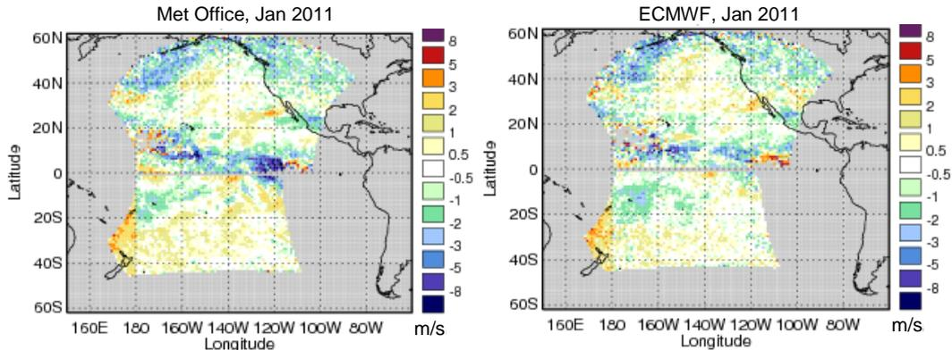
**Figure 41:** Map plots of O-B speed bias for high level GOES-11 IR AMVs in January 2011. Departures versus the Met Office (left) and ECMWF (right) models.
