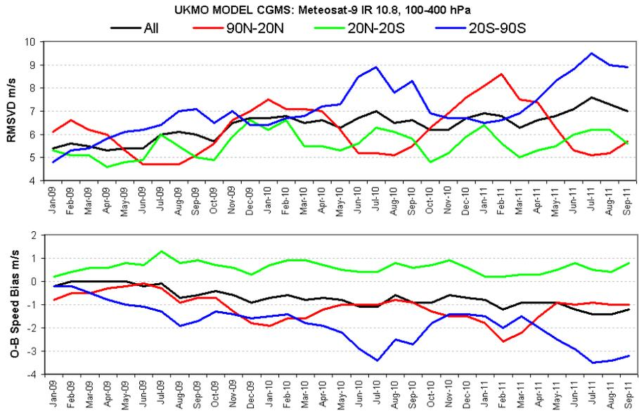
**Figure 29:** Time series of Met Office monthly CGMS statistics for Meteosat-9 high level IR AMVs: root mean square vector difference (top) and O-B speed bias (bottom) for January 2009 to September 2011. Statistics calculated against the Met Office global model background for AMVs with Q11 > 80% (with first guess).
