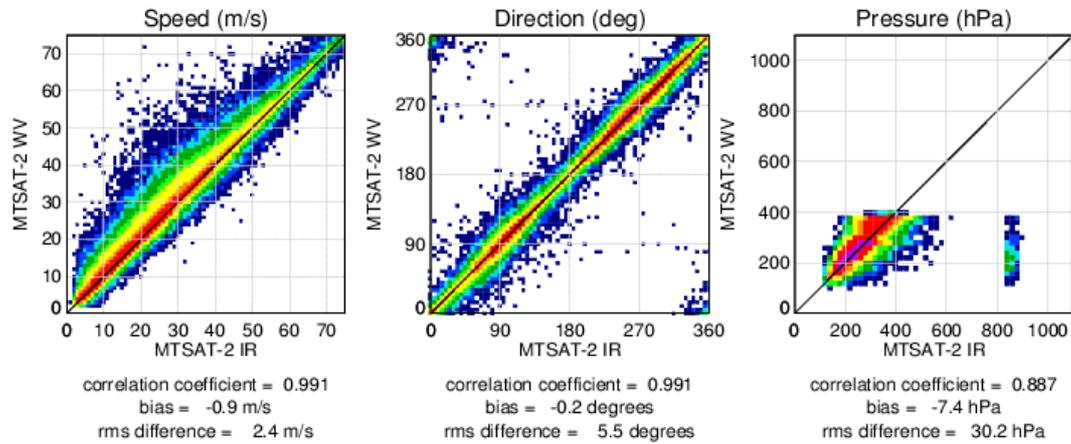
**Figure 39:** Speed, direction and pressure density plots for collocated MTSAT-2 IR and WV AMVs in April 2011. Collocated observations are within 10km and 10 minutes.
