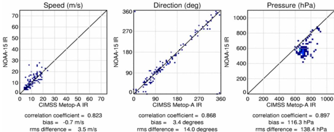
**Figure 6:** As per Figure 5 but this time filtering collocations for Metop winds assigned to cloud base and NOAA-15 assigned to cloud top. 158 matches.
