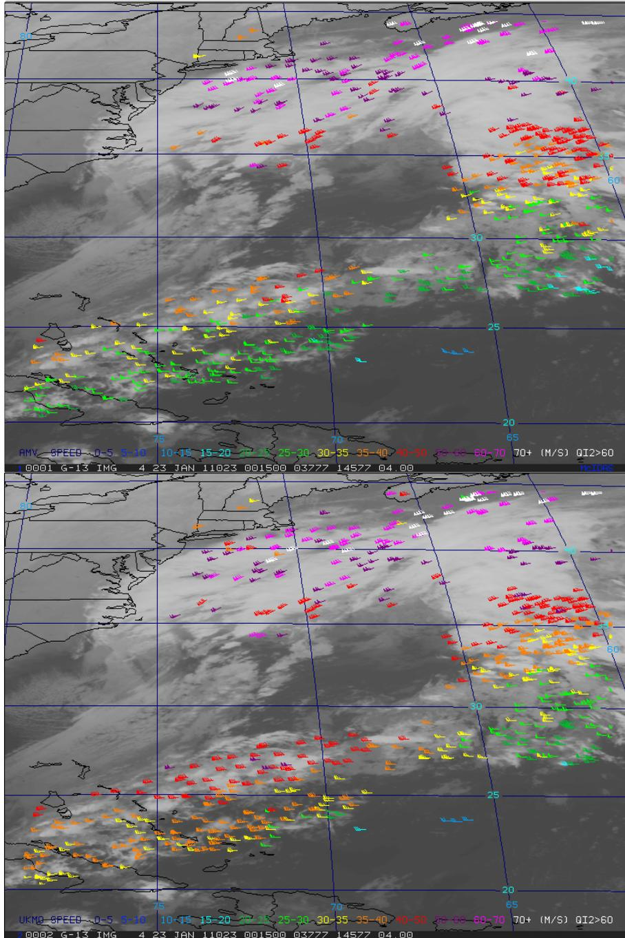
**Figure 32:** McIDAS visualisation of GOES-13 IR10.7 imagery at 0015z off the East Coast of the US. Overlays of GOES-13 IR 10.7 AMVs (top) and collocated Met Office model winds (bottom) have been plotted for high level winds with QI2 > 60. A long barb represents 5 m/s and a pennant 25 m/s.
