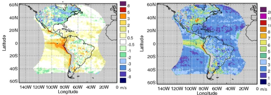
**Figure 10:** Map plots showing mean O-B speed bias (left) and root mean square vector difference (right) for the experimental hourly GOES-13 visible AMVs. Data plotted for November 2011 compared with the Met Office model background.
