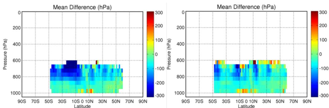
**Figure 11:** Zonal plots of mean difference between GOES-13 visible assigned pressure and model best-fit pressure for the 2011 operational stream (left) and the experimental hourly stream (right). Data is for period November 2011 and observations over sea only.
