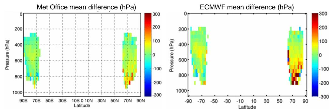
**Figure 46:** Zonal plots of the mean difference between assigned AMV height and the model best-fit pressure height estimate: Met Office (left) and ECMWF (right) models. Statistics are for NESDIS MODIS Aqua IR winds assigned using the EBBT method, over land in February and March 2010.
