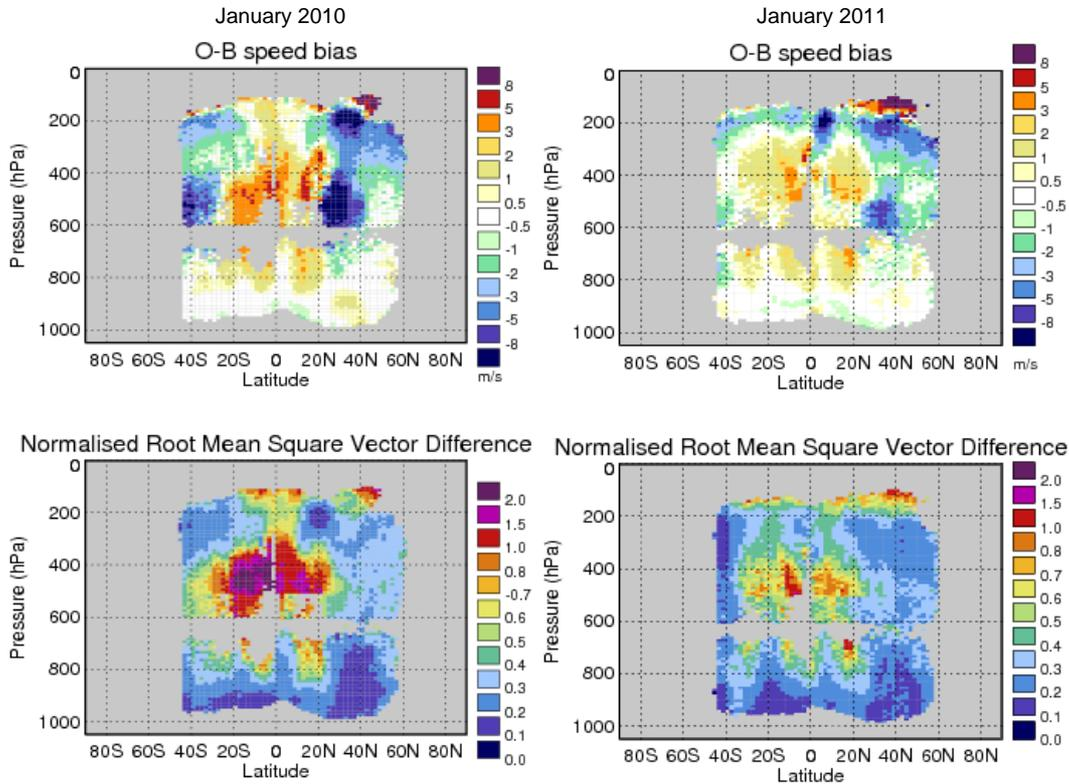
**Figure 24:** Zonal plots of O-B speed bias (top) and normalised RMS vector difference (bottom) for unedited GOES-11 IR AMVs for January 2010 (left) and January 2011 (right). Data compared with the Met Office model background.
