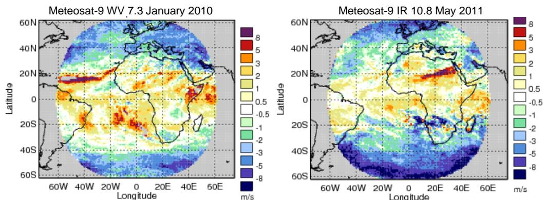
**Figure 33:** Map plots of O-B speed bias for high level Meteosat-9 WV 7.3 AMVs in January 2010 (left) and IR 10.8 AMVs in May 2011 (right). Data compared with the Met Office global model background.
