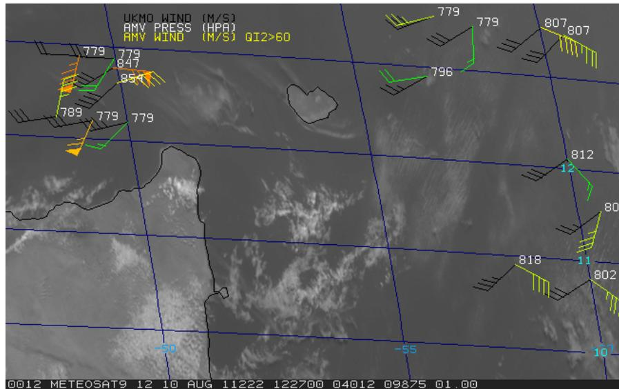
**Figure 23:** McIDAS visualisation of Meteosat-9 high resolution visible imagery at 1227z over the tip of Somalia. Collocated Meteosat-7 visible AMVs (coloured by speed) and Met Office model winds (black) have been plotted along with the AMV assigned pressure. A long barb represents 5 m/s and a pennant 25 m/s. AMVs extracted at 0900z, 1030z, 1200z and 1330z.
