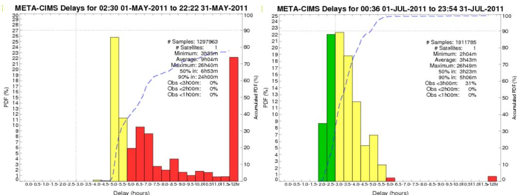
**Figure 2:** Histogram of delay times for CIMSS Metop-A in May 2011 (left) and July 2011 (right) before and after the implementation of the EUMETSAT ADA. Statistics courtesy of Dave Offiler, Met Office.
