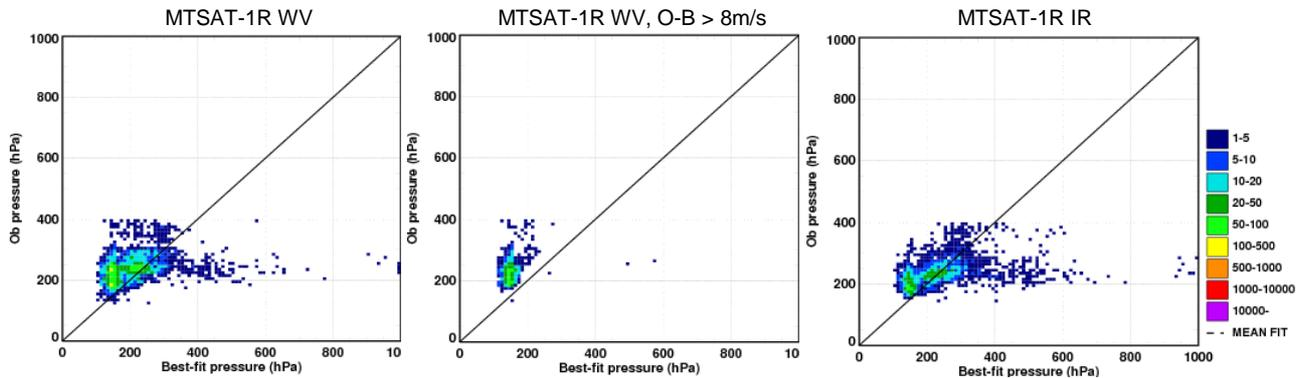
**Figure 37:** Density plots of observed pressure versus model best-fit pressure for MTSAT-1R AMVs valid at 0600 UTC 6 August 2011. Data filtered to a geographical box 10-40N, 120-140E for AMVs above 400 hPa. All WV winds (left), WV winds with O-B speed bias of greater than +8 m/s (middle) and all IR winds (right),
