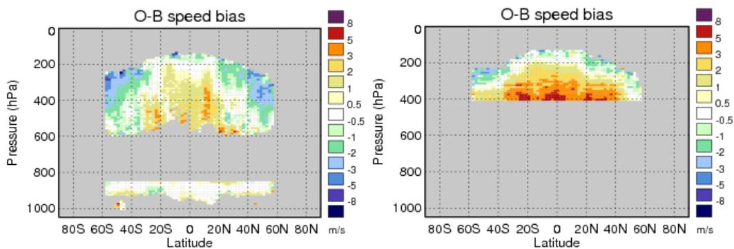
**Figure 38:** Zonal plots of O-B speed bias compared with the Met Office model background for MTSAT-2 IR (left) and WV (right) AMVs for April 2011. Though improved, a slow bias can still be seen in the extra-tropics for the IR data whereas a fast bias is prevalent in the WV data.
