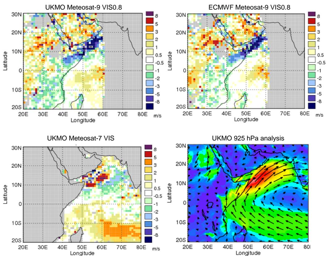
**Figure 17:** Map plots of mean O-B speed bias for Meteosat-9 visible AMVs versus the Met Office (top left) and ECMWF (top right) model backgrounds for August 2011. Also shown is the mean O-B speed bias for Meteosat-7 visible AMVs versus the Met Office model background (bottom left) and the mean Met Office model analysis wind vectors at 925 hPa for August 2011 (bottom right).
