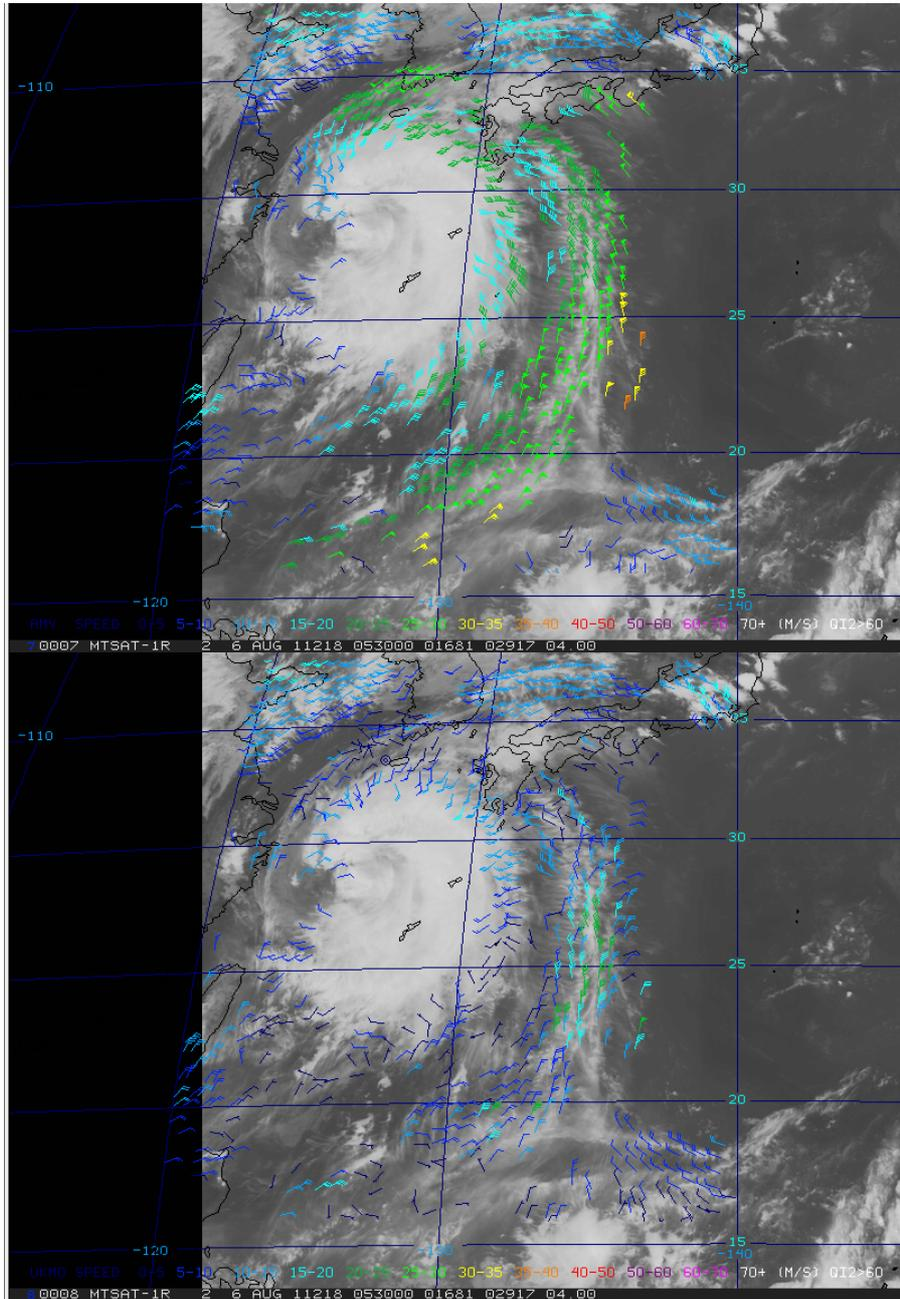
**Figure 36:** McIDAS visualisation of 4 km resolution MTSAT-1R IR10.8 imagery at 0530z, 6 August 2011. Overlays of MTSAT-1R cloudy WV AMVs (top) and collocated Met Office model winds (bottom) have been plotted for high level winds with QI2 > 60. Winds extracted at 0530z only. A long barb represents 5 m/s and a pennant 25 m/s.
