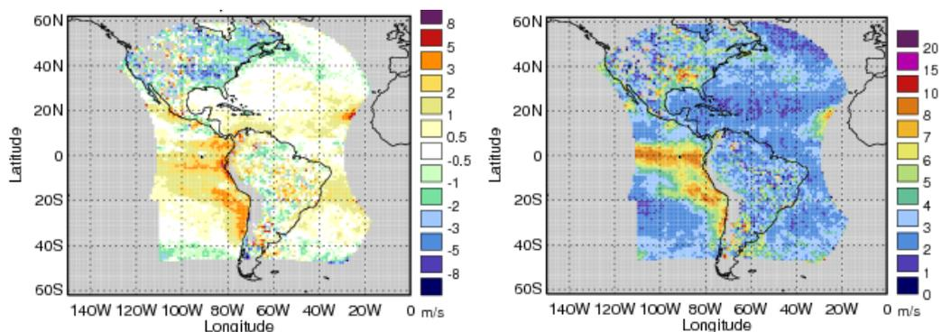
**Figure 8:** Map plots showing mean O-B speed bias (left) and root mean square vector difference (right) for the operational GOES-13 visible AMVs. Data plotted for November 2011 compared with the Met Office model background.
