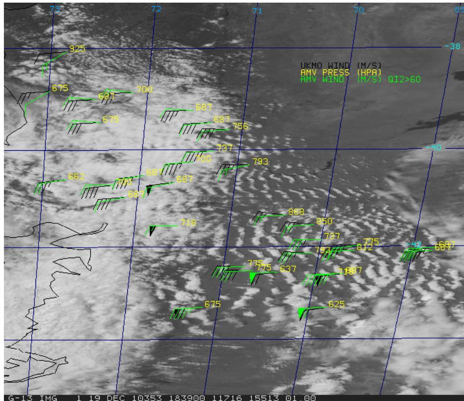
**Figure 14:** McIDAS visualisation of GOES-13 visible imagery at 1839z over Chile/Argentina. Collocated GOES-13 visible AMVs (green) and Met Office model winds (black) have been plotted along with the AMV assigned pressure. A long barb represents 5 m/s and a pennant 25 m/s.
