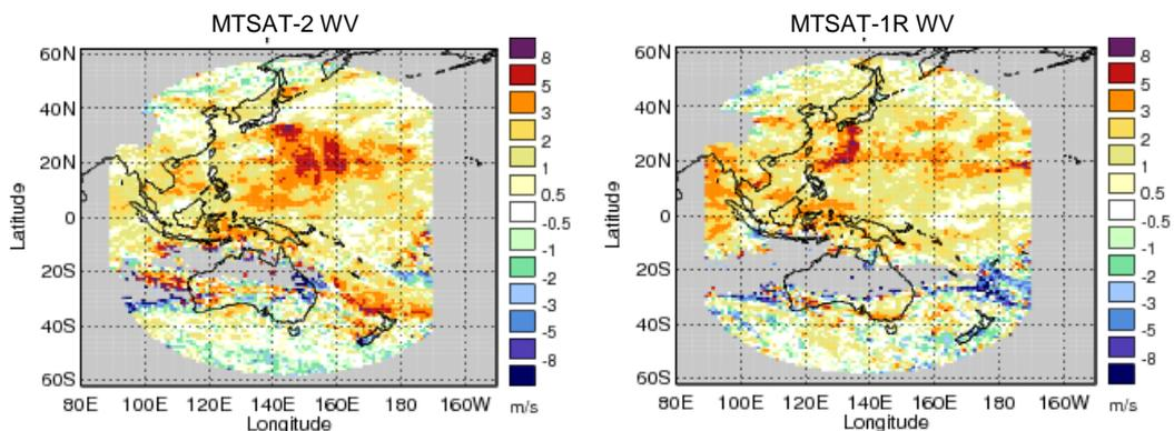
**Figure 34:** Map plots of O-B speed bias for high level MTSAT-2 WV (left) and MTSAT-1R (right) WV AMVs in August 2011. MTSAT-1R was used as backup from 3-15 August inclusive, MTSAT-2 during the remainder of the month.
