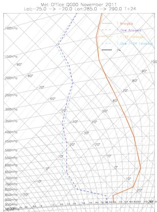
**Figure 9:** Met Office global model tephigram for November 2011 showing the mean temperature (red) and dew point analysis (purple) for a latitude/longitude box 20-25 S, 70-75W.
