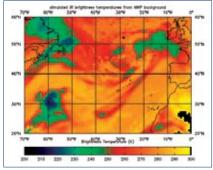
Simulated Meteosat water vapour image using the RTTOV radiative transfer model and NWP fields
