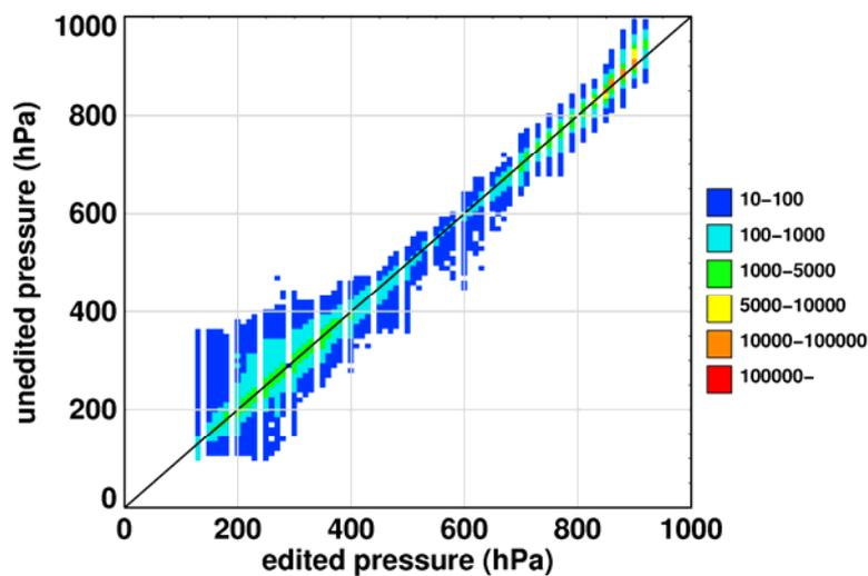
**Figure 5:** Density plot of unedited pressure against edited pressure for one day of GOES-10 and GOES-12 winds produced at NESDIS.
