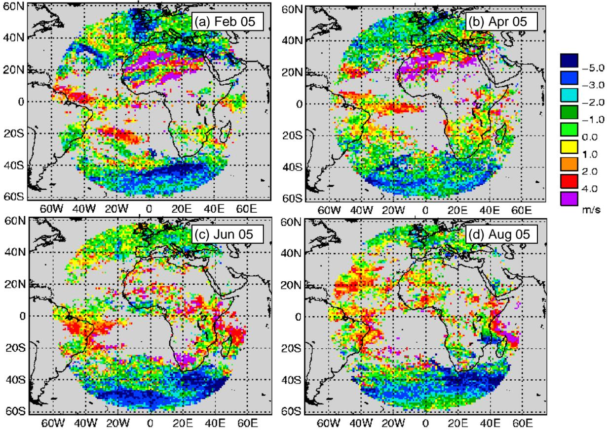
**Figure 23:** O-B speed bias plots for Meteosat-8 IR mid-level (400-700 hPa) winds compared with the Met Office model background for (a) February 2005, (b) April 2005, (c) June 2005 and (d) August 2005. Notice the fast bias (pink) over the Sahara region in February and April. Also notice the slow bias (dark blue) at the southern edge of the disc.
